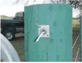
**One-way “CAMEO” vise** – drill 9/16 inch hole in end post for vise
